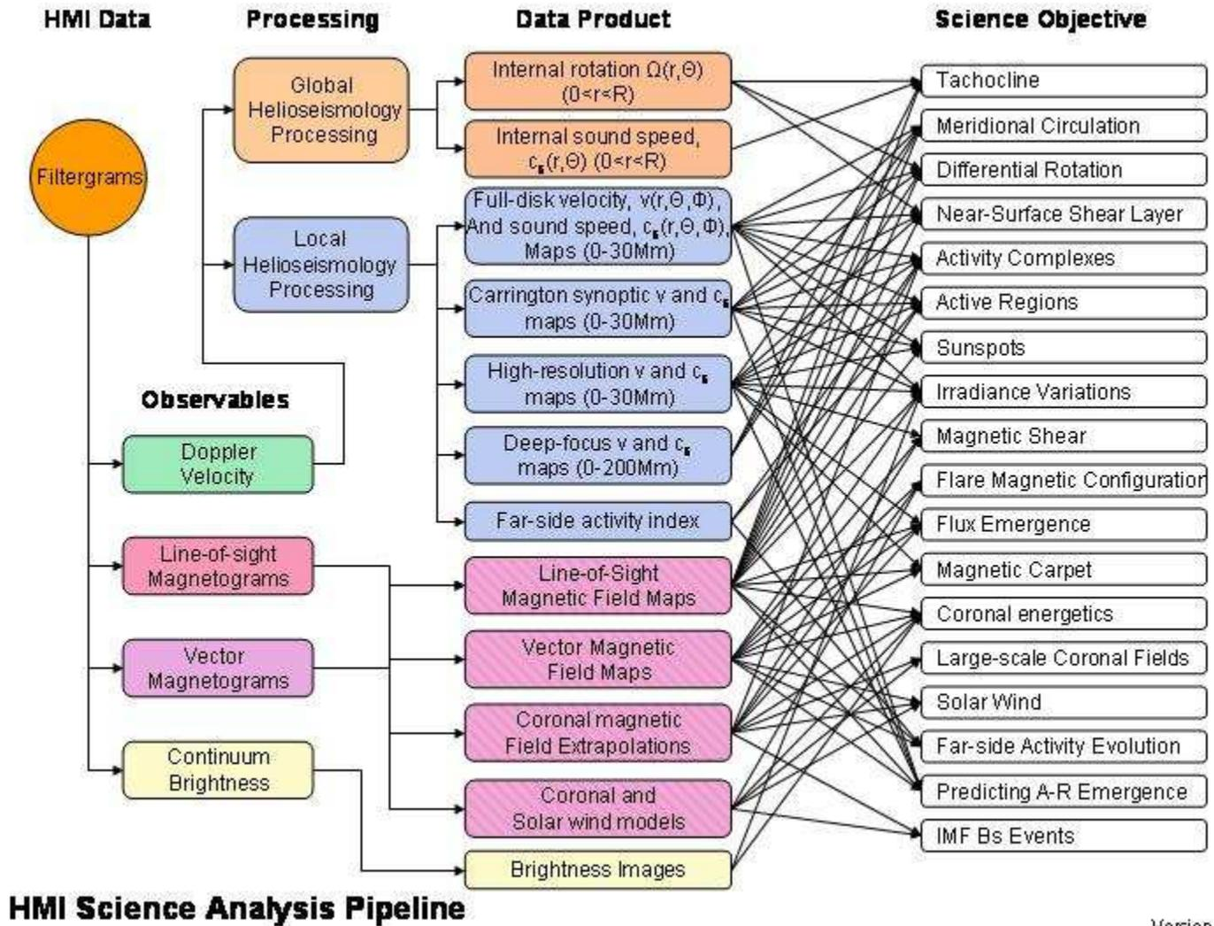
Figure 4: HMI science analysis pipeline flowchart (sourced here), showing how the four main observables are used to create the many data products that support the science objectives of the HMI instrument.
