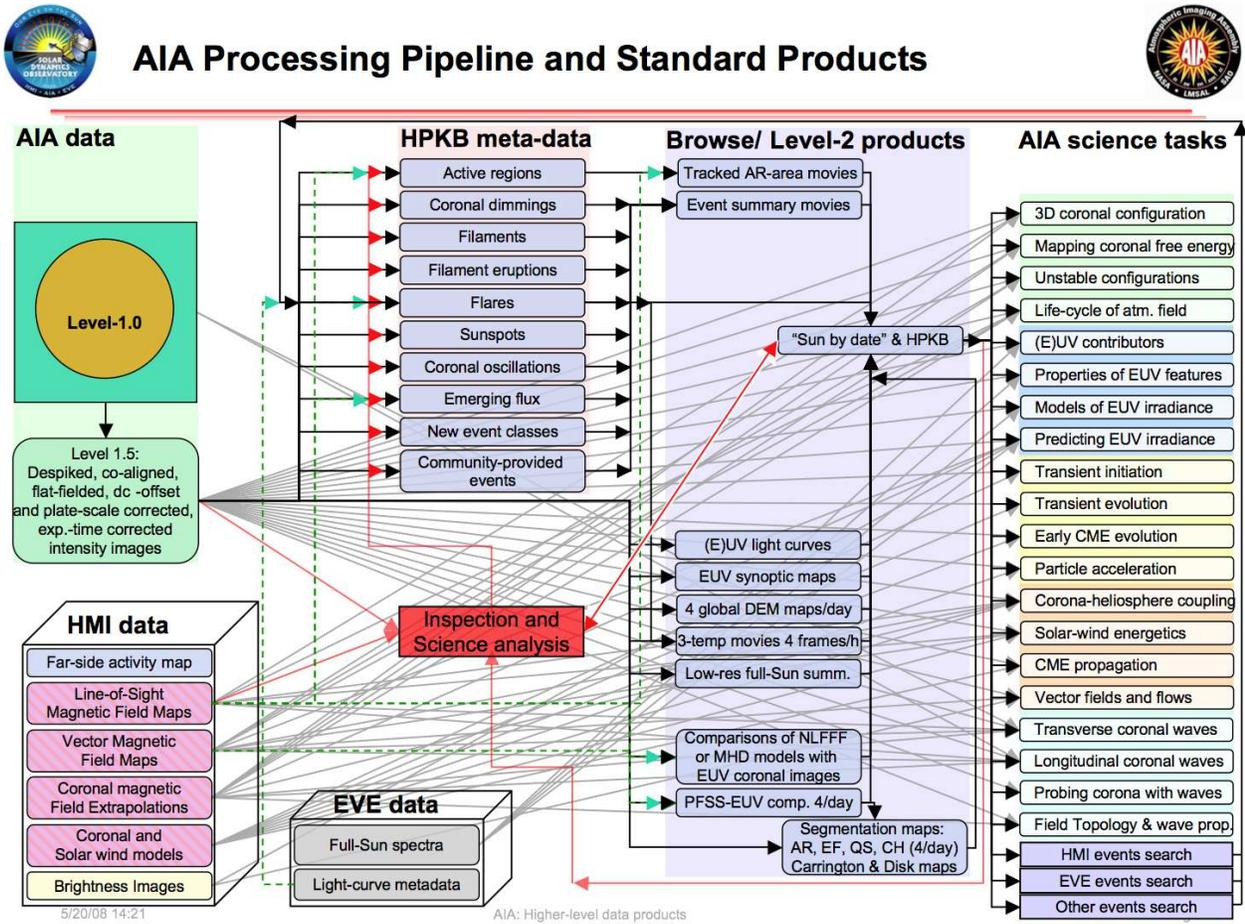
Figure 2: AIA science analysis pipeline, illustrating how the main filtergram data, along with data from EVE and HMI produce the data products that support the science goals of AIA. Note that AIA Level-1.5 data are *not* exposure-time corrected (as is incorrectly indicated in the figure).
